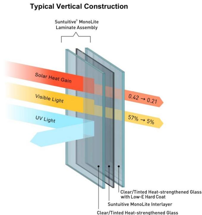
Powered by sunlight, Suntuitive MonoLite dynamically transitions from light to dark in response to solar heat without any wires or controls and installs the same as traditional glass, offering performance unlike any other single pane glass, while still fitting glazing pockets as small as 6.3mm (¼").
