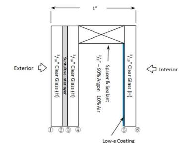
Suntuitive interlayer is laminated between two pieces of heat strengthened or tempered glass and placed into an insulated glass unit (IGU) with a low emissivity coating. A warm edge spacer is also recommended.
